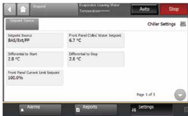
Figure 52. Example equipment settings screen (Chiller Settings shown)
