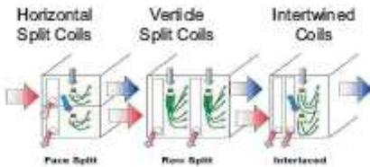
FIG. 2 -EVAPORATOR COIL TYPES
