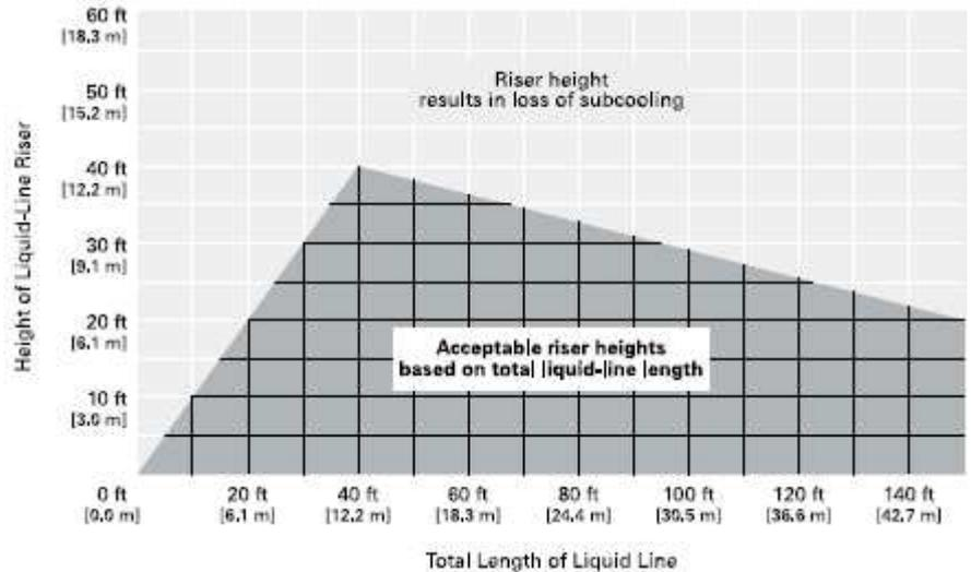
Riser height limitations defined in this chart assume that the liquid line contains 10 elbows. The effect of additional elbows varies based on the specific characteristics of each installation.
