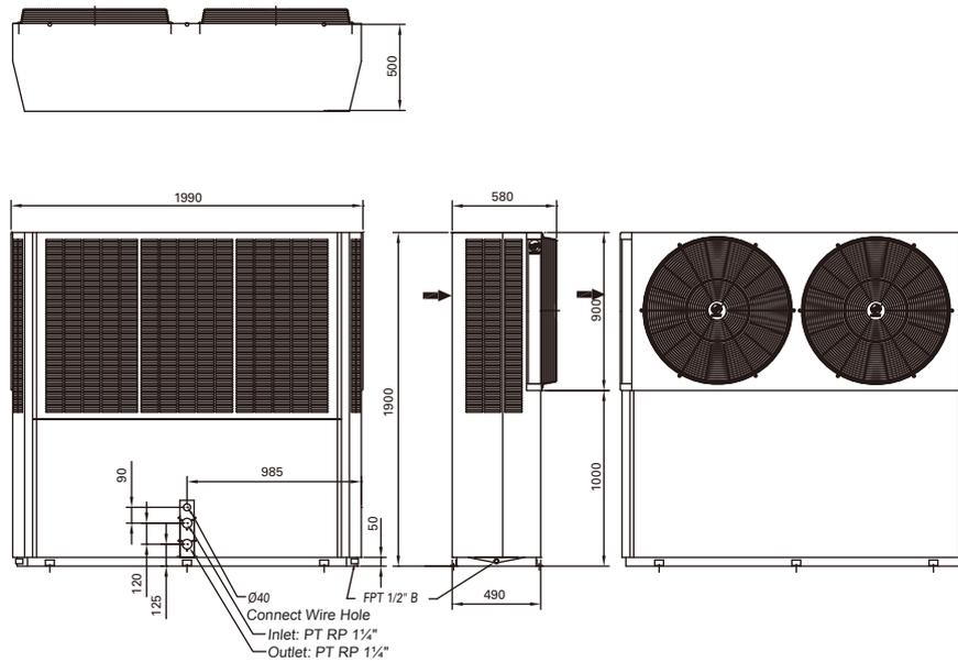
Note: Water Connection (FPT) for CGAR/K2005R is PT RP 1-1/2".
