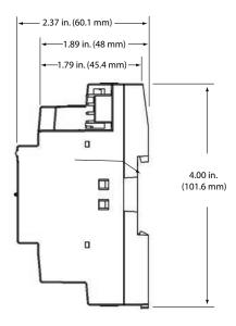
\*DIN Standard 43 880, Built-in Equipment for Electrical Installation. Overall Dimensions and Related Mounting Dimensions.
